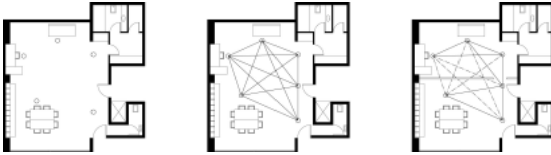
Figure 1: The plan of a setting, with behavioral micro-settings marked. The implications of adding a partition represented as transformations of an underlying connectivity graph
